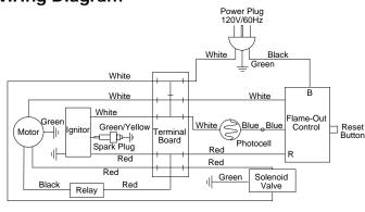
Figure 26 - Wiring Diagram
